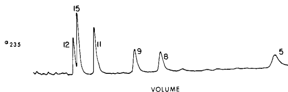
Figure 1. HPLC chromatogram of oxidation products from 0.2 M arachidonic acid in 97% cyclohexadiene/3% benzene. HPETE isomers are indicated on the chromatogram. LC conditions are as described in the text.
